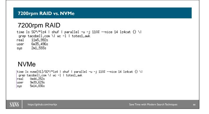
The RAID I used is five 7200rpm 2TB drives in RAID 5. This is meant to be representative of an Enterprise configuration.
