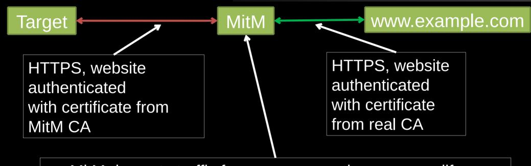
MitM decrypts traffic from one connection, may modify or record the plaintext, re-encrypts it with the key for the other connection, then forwards it
